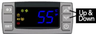
To view the "High Temp" recorded by the cooling unit, press the "Up" button once.
