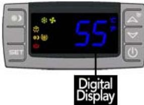
The temperature displayed on the control indicates the real-time air temperature as measured by Probe 1 (P1) located behind the front grill of the cooling unit, or the temperature (air or liquid) being measured by the bottle probe (the bottle probe overrides P1).
