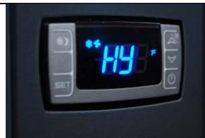
**TEMPERATURE DIFFERENTIAL:** The factory preset for this setting is “4” without a bottle probe, and “1” with a probe.
