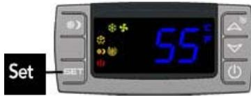
The cooling unit is factory preset with a Minimum Set Point of 58°F and a Temperature Differential of 4°F. This means that the cooling unit will turn on when the display rises above 62°F (58°F + 4°F), and turn off when the display falls below 58°F.
